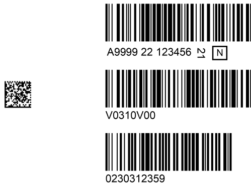
Figure 1 Comparison of 2-D and Linear Bar Codes
